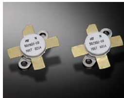
●200-Watt Version Utilizes Push-Pull SD2931 Devices
