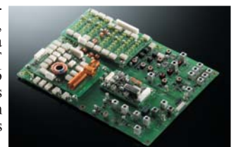
RX Unit (Showing the VRF and BPF Units)
